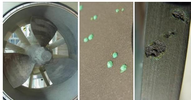
**Figure 4.** Kaplan runner enclosed by the runner ring (left), with numerous green tubercles (middle) covering pit-like metal loss of several mm diameter (right).
