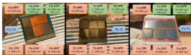
Figure 3. Image of irradiated ink with different values of laser irradiance and different types of scanning (a) Cu-50, (b) Ni-50 and (c) Co-50 samples.
