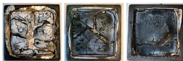
Figure 3. Reference (left), sample with commercial flame retardant (center) and sample with synthesized flame retardant (right).
