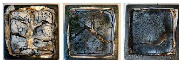
Figure 3. Reference (left), sample with commercial retardant (center) and sample with synthesized retardant (right).
